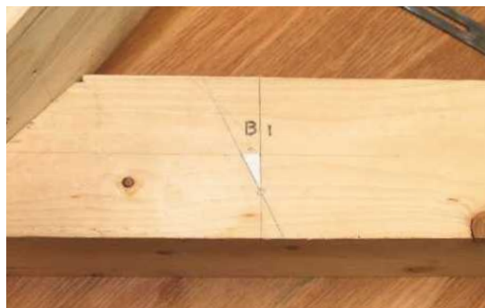
▲ Pic.4 Here a paper triangle has been drawn using Pythagoras' Theorem and it is placed on the actual location where a layout line needs to be drawn, just below point (B1). This makes it easier to visualise how the layout lines relate to the 3D model. One of our group drew up a CAD version of the model, which could be rotated and all the main angles were shown in different coloured triangles
